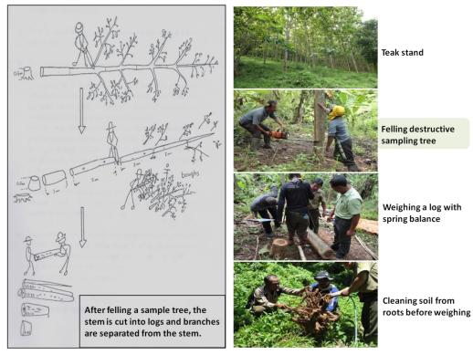
Figure 2. Procedures to measure tree bio-mass
